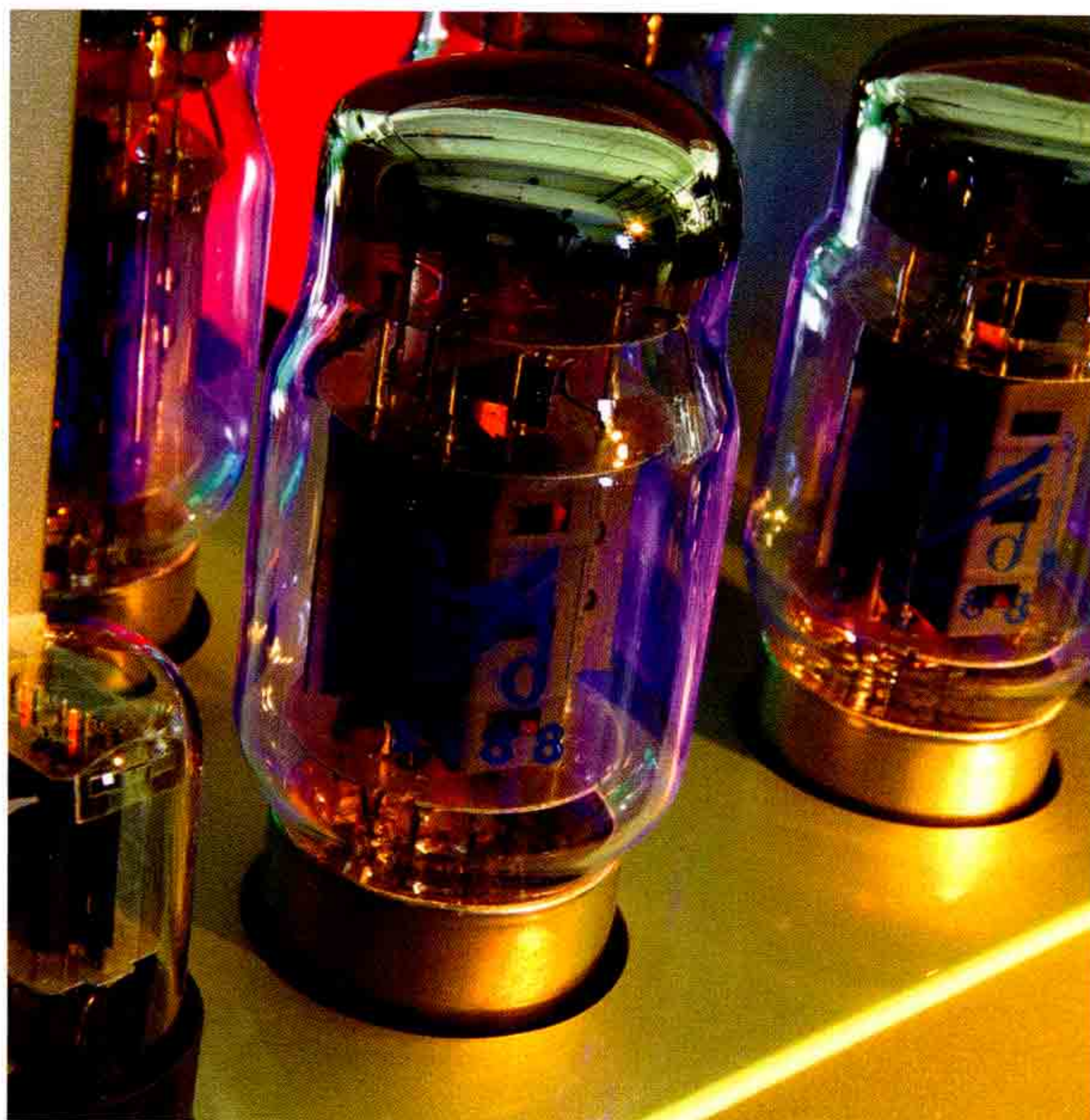
ABOVE: Two pairs of KT88 'beam power tetrodes' are employed in a dual push-pull output configuration
