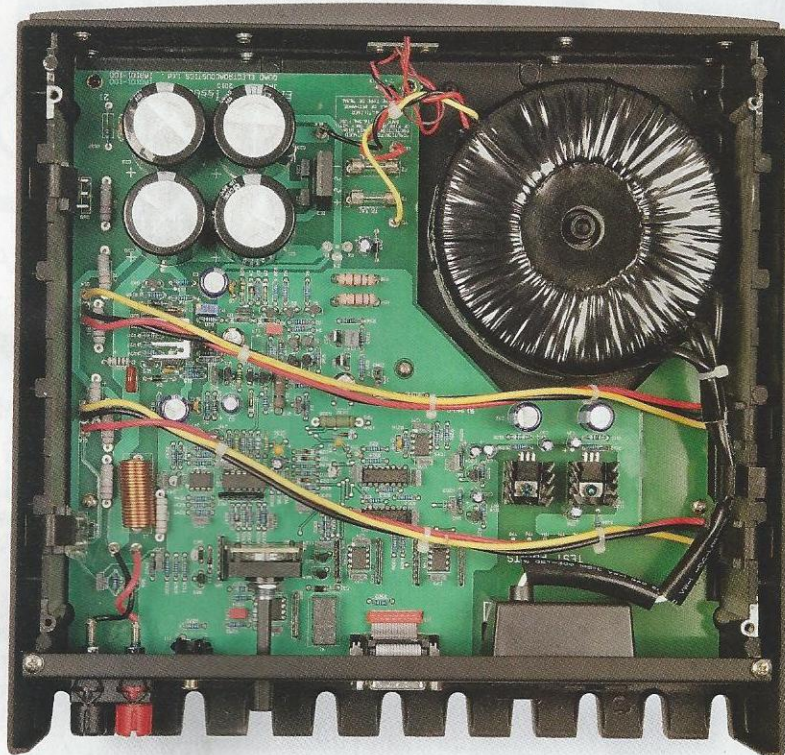
ABOVE: Mono power amp houses large toroidal transformer for power supply, and large mother board; binding posts (lower l/h corner) accept bare wire or bananas
