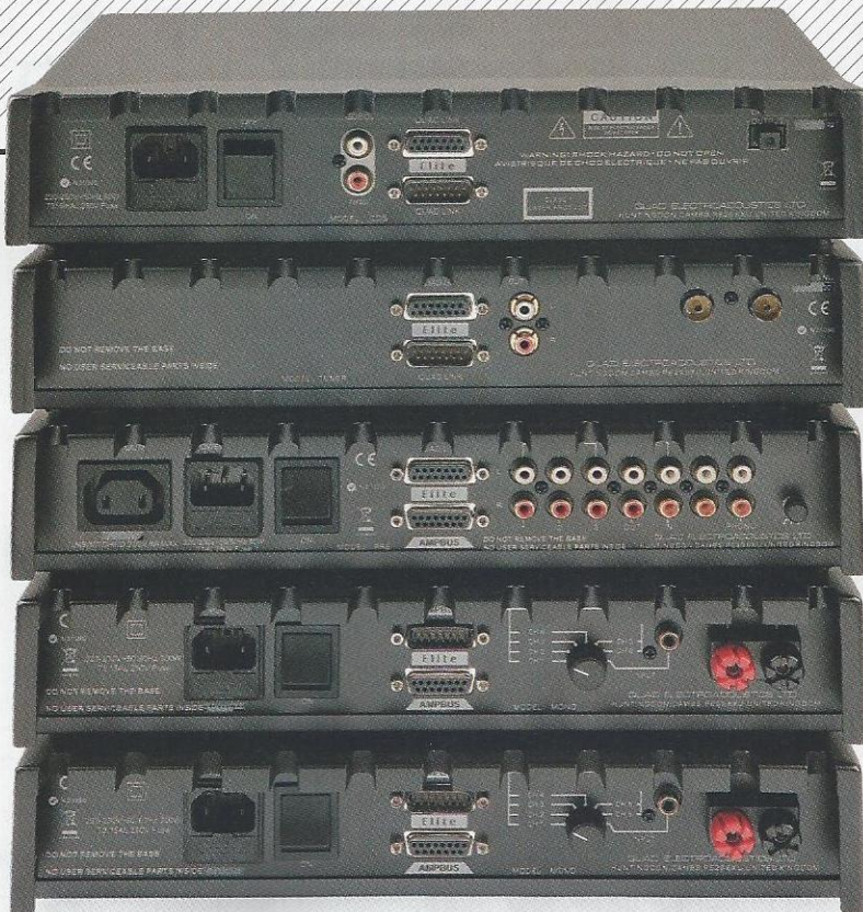
ABOVE: The use of the Quad Link ribbon-cable connections eliminates the need to employ conventional interconnects and improves operational control of the system
