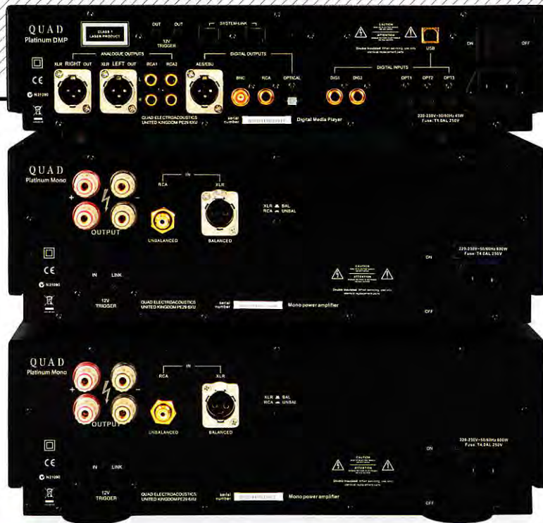
ABOVE: All units are clearly labelled and fitted with good-quality connectors. Note balanced XLR connection for pre-to-power, and four types of digital outputs and six digital inputs, including USB, on the back of the DMP. The Monos facilitate bi-wiring
