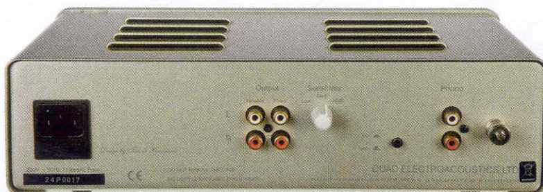
ABOVE: Here a small push button selects standard MM or MC gain, while the knob near the centre gives high, low, or medium gain options in either mode
