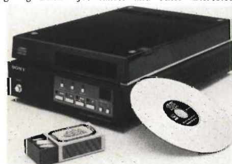
Sony prototype Compact Digital Disc player, with disc and a matchbox to show the small dimensions.
