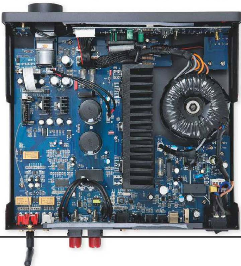
RIGHT: A single toroidal transformer (with multiple taps) feeds independently-regulated supplies for the (integrated) Class A/B power amp and DAC section. Note motorised volume
