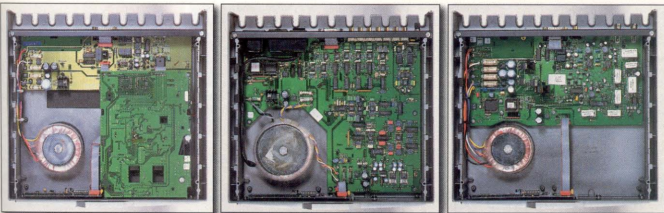
Inside (from left to right) the 99 CD player, pre-amplifier and tuner. Servicing should be easy, with access by simply removing the base plate
