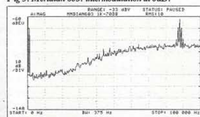
Fig 4. Meridian 603: ultrasonic spurs associated with -70dB 1kHz tone, to 100kHz.
