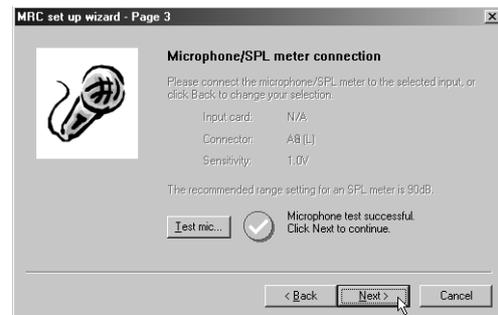
If the test did not complete successfully check the SPL meter or microphone connections and the input card and connector settings and try again. For more information about problems with the microphone test see *Troubleshooting*, page 48.
